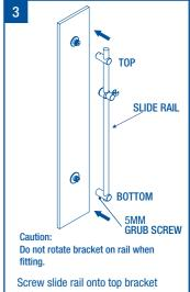
Slide bottom bracket onto slide rail (grub screws to bottom).
